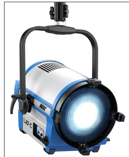
**L10-C** Color temperature, tint and hue can be continuously adjusted from 2,800 K to 10,000 K, between full plus or minus green and RGBW colors.
