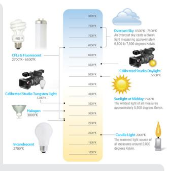
Most common lighting conditions produce light in the temperature range from around 2,000K to 8,000K. In practical terms this usually means selecting lights, gels and filters which are most appropriate to the prevailing light or to create a particular colour effect.
