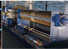
Whether low-speed or high-speed, high-capacity Vortek hoists are used in facilities of all sizes – from high school gyms to professional arenas. Vortek hoist technology combined with the principle of single point of failure prevention design makes Vortek Scoreboard hoists the standards in the arena rigging industry. Custom hoists are also available to accommodate any kind of lift capacity or mounting option imaginable.
